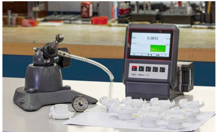
The non-contact characteristic of air gaging makes it particularly useful for checking soft, highly polished, thin-walled or otherwise delicate material.
